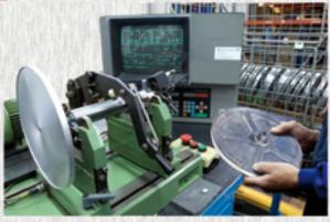
2. All our discs are individually balanced according to the strict ISO-1940/2953 norm, the same norm used, for example, to balance the turbines of the jet planes. The tolerance allowed is 0.1 g/mm. The large mass of the disc (large angular momentum) and a thorough balancing result in a surprisingly smooth operation.
