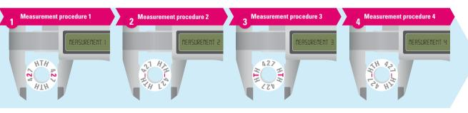
Measure the diameter of the sintering ring at the middle number (example of the sintering ring).
