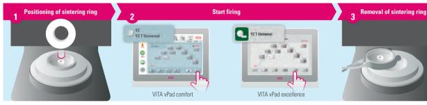
Place the sintering ring without sintering beads in the center of the sintering tray\*.
