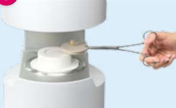
Remove the firing tray and restoration
