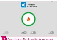
2 2nd phase: The icon lights up green. The heating/cooling phase starts.
