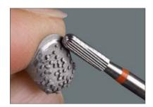
The framework is prepared using cross-cut milling tools in accordance with the specifications of the alloy manufacturer. Surfaces not to be veneered, in particular occlusal surfaces, are polished with rubber polishers.
