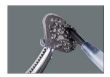
PRE OPAQUE is applied onto the framework with a disposable brush.
