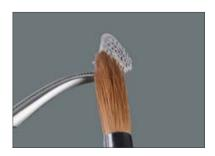
The metal framework is cleaned after sandblasting. Use only dry compressed air (with water separator) or a clean dry brush for cleaning.
