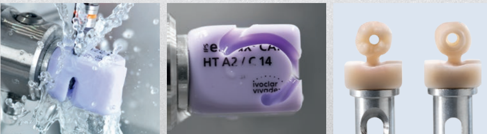
"Carving Mode" - excess material is being cut off as a whole
