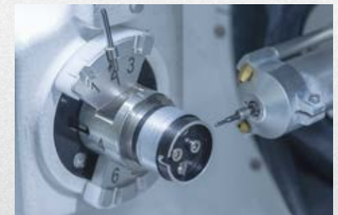
Precision calibration ensures correct alignment of the abutment and implant connection geometry
