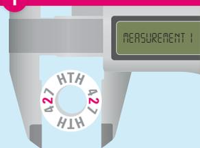
Measure the diameter of the sintering ring at the middle number (example of the sintering ring).
