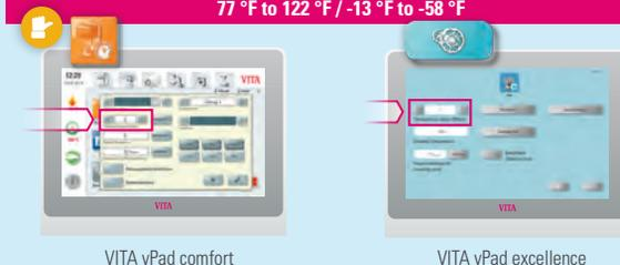
Correct the oven temperature. Insert the difference value in the "temperature adjustment (offset)" field\*.
