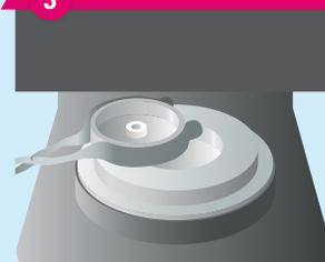
Remove sintering ring and measure with caliper.
