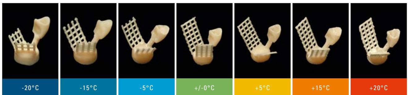
Figure 4: VITA AMBRIA grid retentions and crown at different firing temperatures
