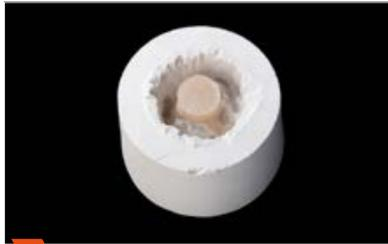
**4** Perform rough divestment with Al<sub>2</sub>O<sub>3</sub> (50 µm grain size) at a pressure of 4 bar.
