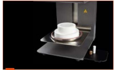
**3** Prepare a cold press pellet and a cold plunger in the required shade.
