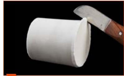
**3** Break the edges of the investment ring without allowing investment material to fall into the channel.
