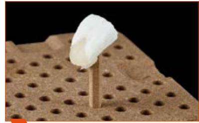
**3** Fix veneer on the firing tray with VITA Firing Paste.
