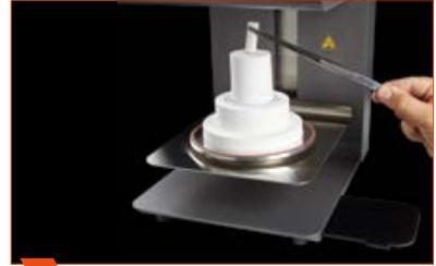
**6** Place the disposable press plunger with the point up on the pellet.
