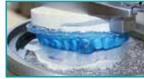
22. Now execute the second thermoforming process. As soon as the foil is adapted, close the Occluform. Allow to cool completely. Uncover all spacers before taking the splints off the model. Thereto, **carefully** grind through the plate ...
