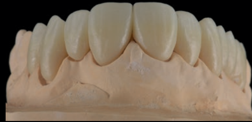
Figure 1: KATANA™ Zirconia YML 4-unit and 6-unit bridges after milling and sintering. A natural vestibular surface texture plays a decisive role in the creation of aesthetic monolithic restorations.
