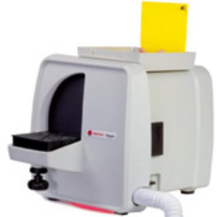
Besides, the Mulhacén trimmer and the Mestra R-080087 conform a perfect couple: they fit perfectly into the lab and take a minimum space. They are connected by very flexible threaded couplings, so in most of the cases can be installed by the user himself.
