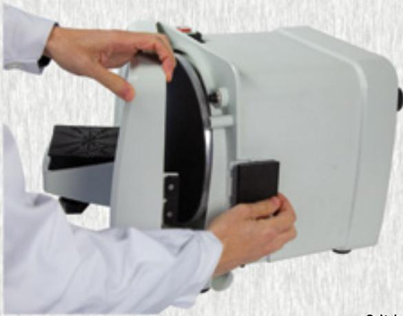
2 You can access the abrasive disc easily through the door fitted with a quick opening hinge. You can open and close the lid in a few seconds. The disc maintenance, cleaning and replacement are surprisingly simple.
