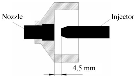
If the nozzle came loose, glue it to its holder with cyanoacrylate. The nozzle should be level with the inner surface of the nozzle holder, to make sure that the distance from the injector to the nozzle is 4.5 mm and the Venturi effect takes place.
