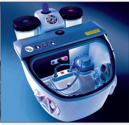
When talking about savings, we shouldn't just focus on the acquisition cost of the product. You also have to take into consideration maintenance and, above all, savings on consumable parts. Eclipse sandblasters have quick-release valves that, after releasing the pedal, stop the flow of sand in just a fraction of a second. This system not only saves sand, but it also makes the machine significantly safer, as the tank is completely de-pressurised.
