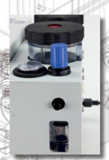
As for the unit's maintenance, all the blasting system can be dismounted quickly, easily and with no tools to solve minor blockages. Thanks to a practical window, the level of condensed water in the pressure regulator filter can be easily seen. This liquid is drained automatically. The silencing filters and the pressure gauge filters should be replaced only once a year (with a normal professional use).
