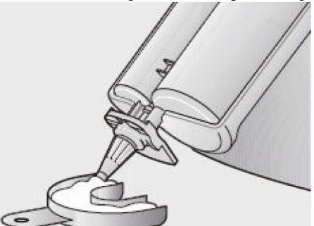
9. Finish injection and press back button (3) to release the cartridge before removing.
