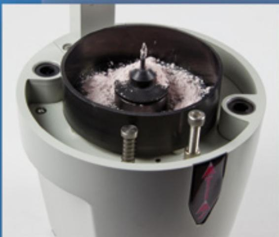
If we now consider the dust produced during the operation, we believe that cleanness has to be another key point when designing a pin drill. In the **Atlas** model the table is easily dismantled without any special tool, and it gives access to an inner container too collect the dirt. Once removed, you can clean the container with water and soap before placing it again.
