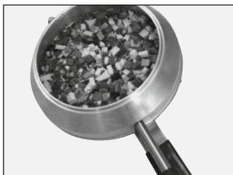
Maintain the active pressing process for at least 3 minutes. If the lamination of the granules is incomplete, turn the plate, if necessary, and carry out a further heating process of 2 min. Go on as described from point 8 on.
