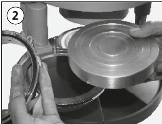
Place the heating pan and the chimney onto the unit adapter and swivel the plate reception into the centre of the unit. At the same time press the plate reception slightly downwards and direct the heating into the heating position. Please observe that the cannellure of the chimney latches into the the heating housing.
