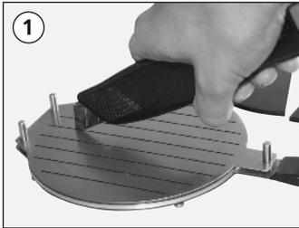
For cutting a hot scalpel or box cutter are recommended. Assort a foil from the stripes according to your wishes.
