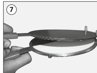
We recommend to put pressing lid onto the guide pin first and to close it transversely afterwards to let escape excess air.
