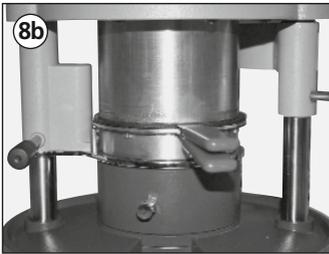
After the pressing procedure has run out move the piston of the unit upwards and remove the combination of heating pan / pressing lid from the unit.
