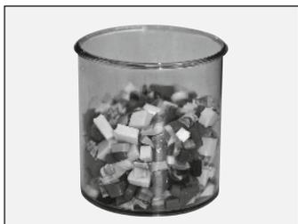
After the first pre-heating time the prepared EVA granules are to be placed into the heating pan, covering the whole bottom of the pan. The second pre-heating time amounts to 2:30 min. Go on as described from point 8 on.
