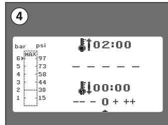
After the first pre-heating time swivel the plate reception outwards and remove the heating pan /chimney from the unit. Then put the cut Drufo-soft stripes into the heating pan according to the desired design and ensuring exact fitting of the cut edges, put on chimney and put everything into the thermoforming unit again, as described in point 3.
