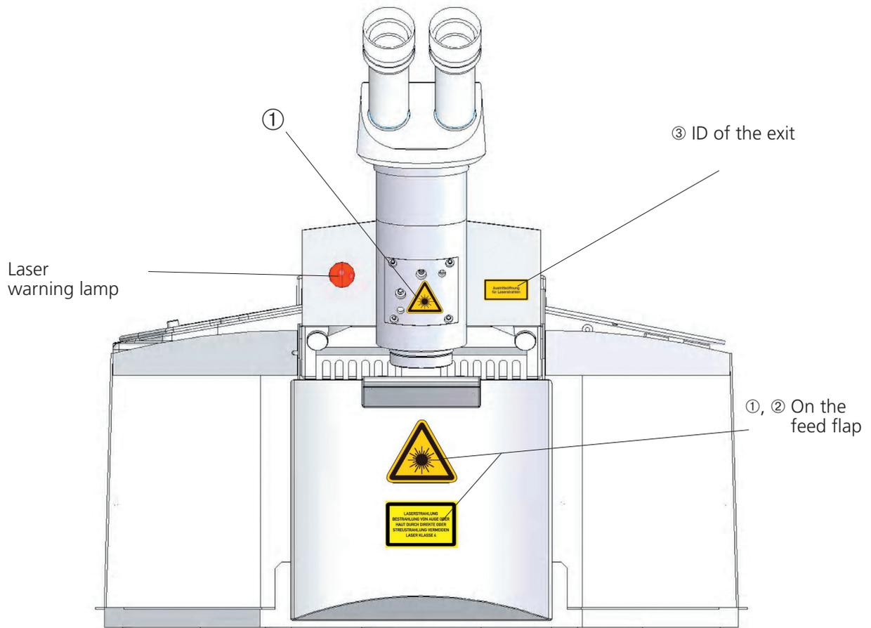
**Fig. 1: Position of the laser warning signs**
