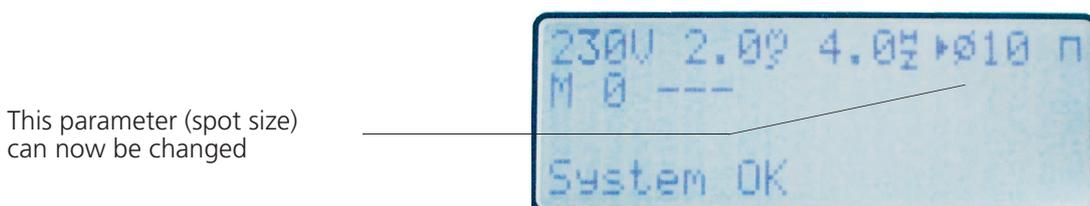
**Fig. 8: In change mode, ► or ◀ identifies the changeable parameter**
