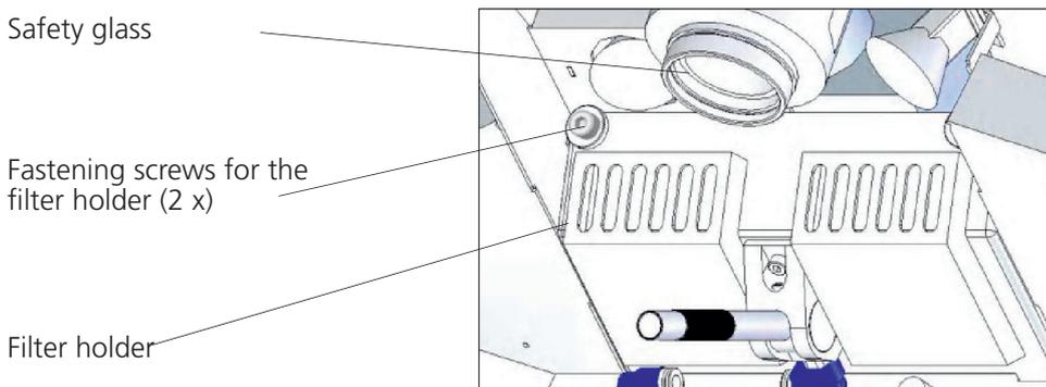
**Fig. 16: Performing maintenance in the working chamber**
