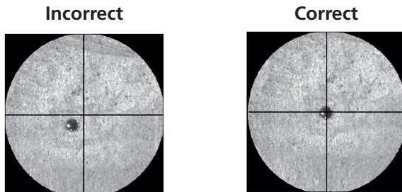
**Fig. 20: adjustment of the laser welding point and reticule**
