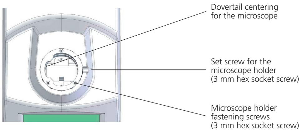
**Fig. 18: Microscope flange (from above)**
