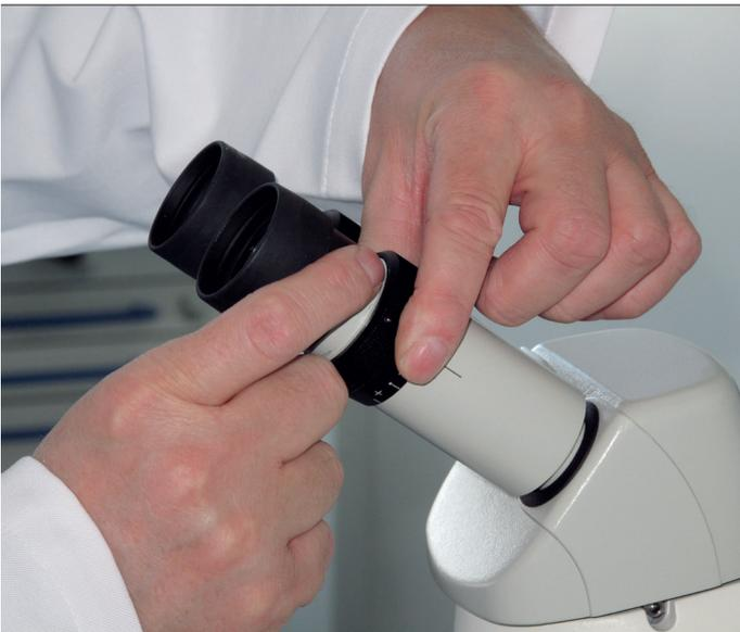
**Fig. 14: Adjust the reticle according to the division scale**
