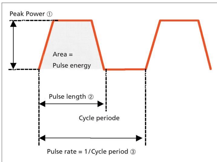
**Fig. 9 : Pulse Parameters ① to ③**
