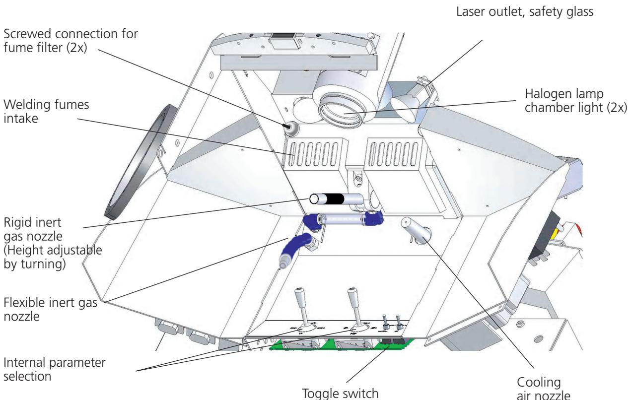
**Fig. 4: View from below into the working chamber**
