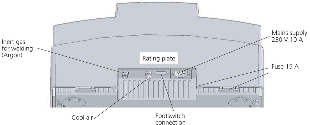
**Fig. 6: Connections on the back of the desktop Compact**
