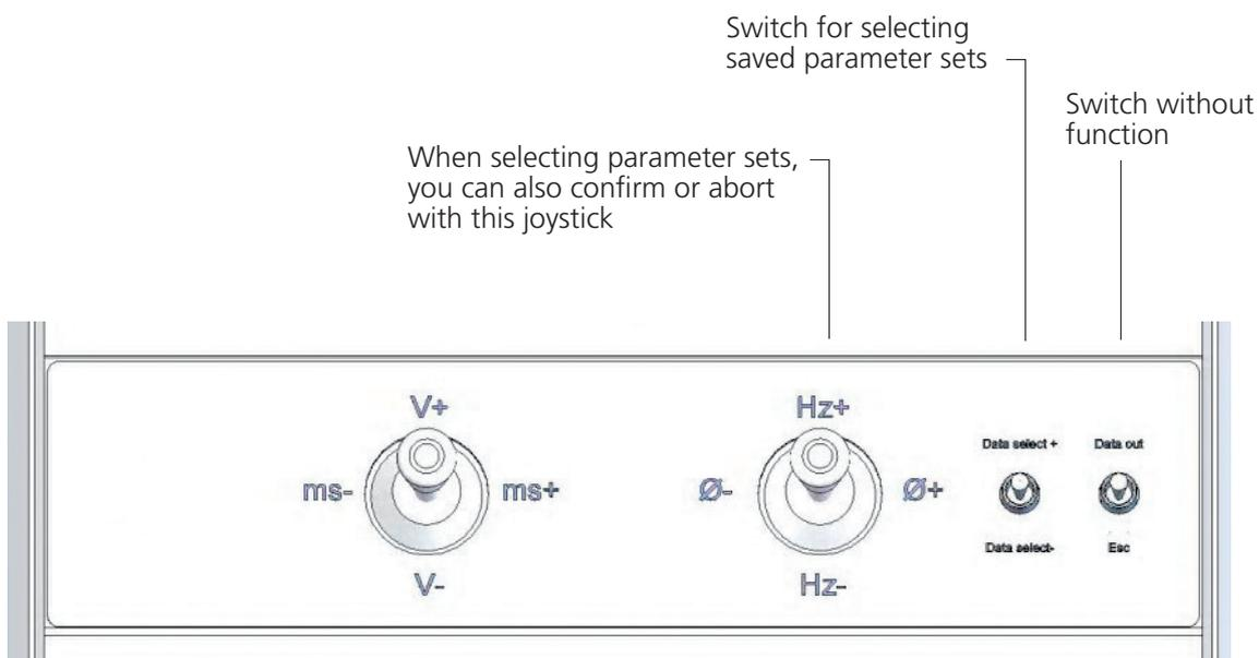
**Fig. 11 : Controls in the working chamber**
