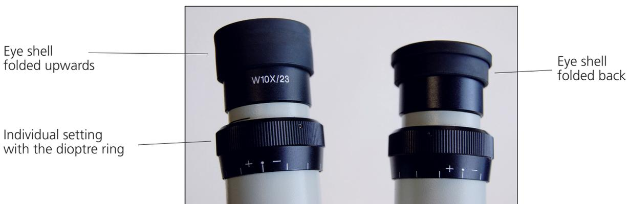
**Fig. 12: Ocular adjustment at the microscope**
