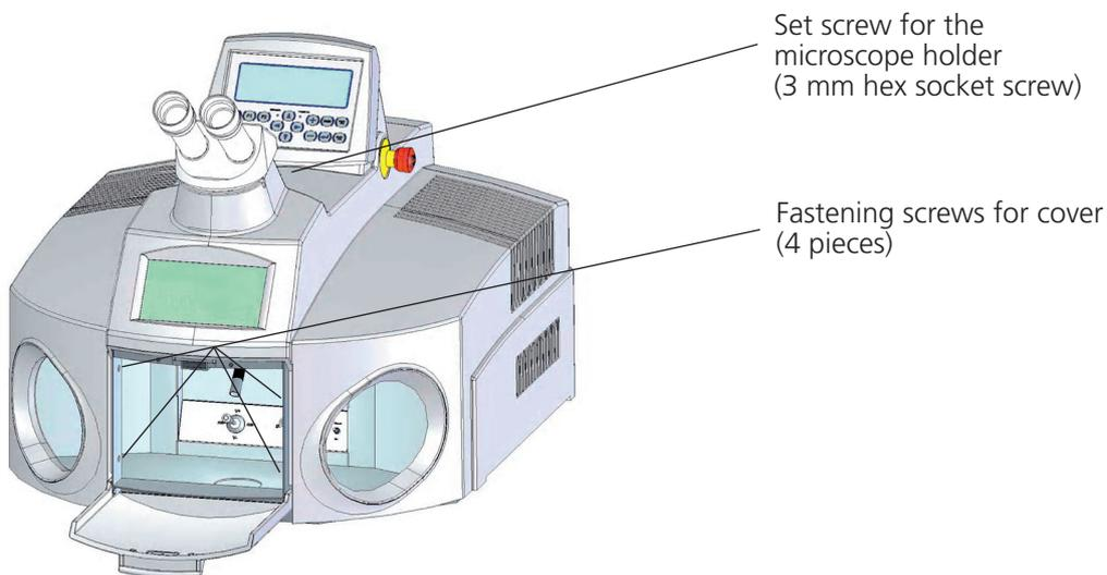
**Fig. 17: Fastening points for the unit cover**
