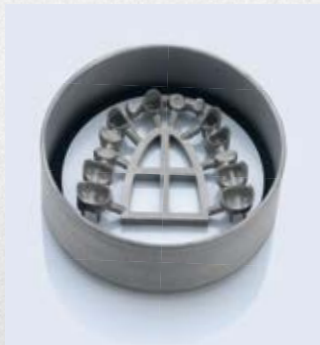
Milled frameworks on Float Sintering Disc in the Ceramill Argovent 2
