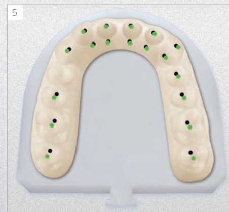
Unrestricted expansion (green) of the plaster due to early separation from the base plate. (Original information = black).
